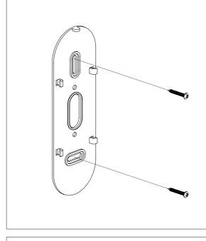
Attach the lamp base to the wall using the orientation displayed below. Always choose screws and plugs that are appropriate for the wall, and ensure the wall cavity is free from electrical cables or piping before commencing drilling.
